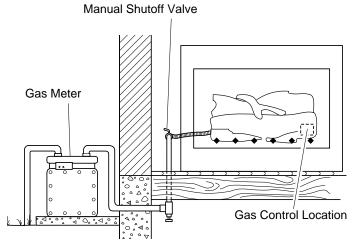
Figure 15 - Checking Gas Joints
